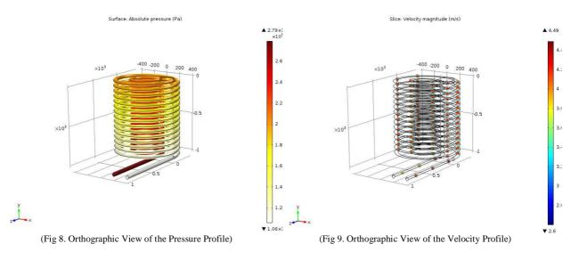
Figure 8 represents the absolute pressure simulation results of the copper coil, maximum pressure is  $2.79 \times 10^{5}$  pascals just slightly above ambient giving a positive flow in the coil and exits the coil at a reduced pressure of  $1.2 \times 10^{5}$  pascals the difference is associated with frictional pipe losses
