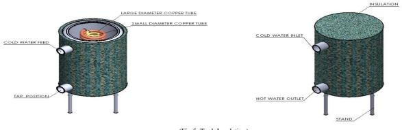
(Fig 5. Tank Insulation)
